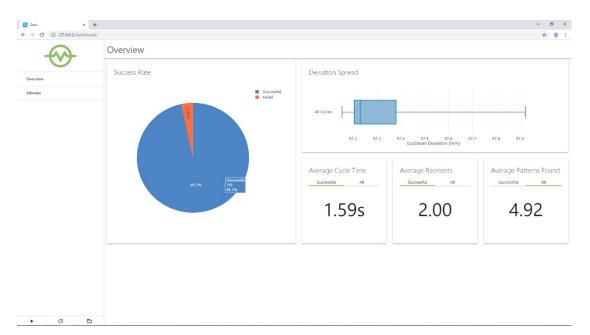
On the workspace overview, users can access these key metrics: cycle success rate, a box-andwhisker plot of the parts deviations from the reference position, average cycle time, average number of reorients, and average number of patterns found. These values give key insight into the speed and variability of their cell. Furthermore, these numbers are lead indicators for any reduced performance of the cell.
