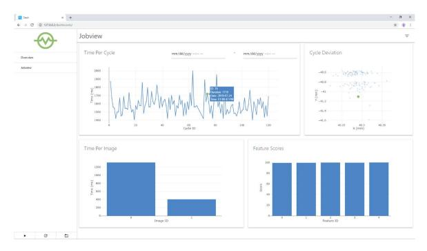
In the job view, users can see individual statistics, like cycle times, deviations in 3 dimensions, cycle time per image, and feature scores. Further filtering can be done on the date range of the data. This allows users to access historical data for inspection and exploration.
